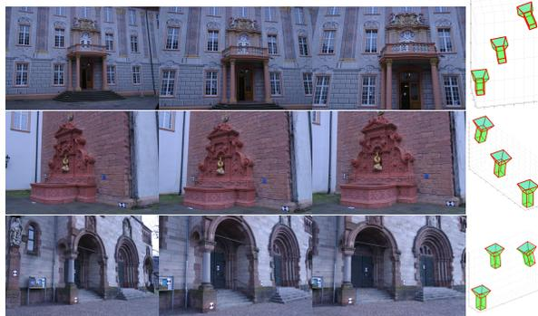
Figure 8. Trifocal relative pose estimation for additional cases from the EPFL dataset. For each row, image triplets samples are shown. The estimation results are shown on the right. Ground truth poses are in solid green and estimated poses are in red.
