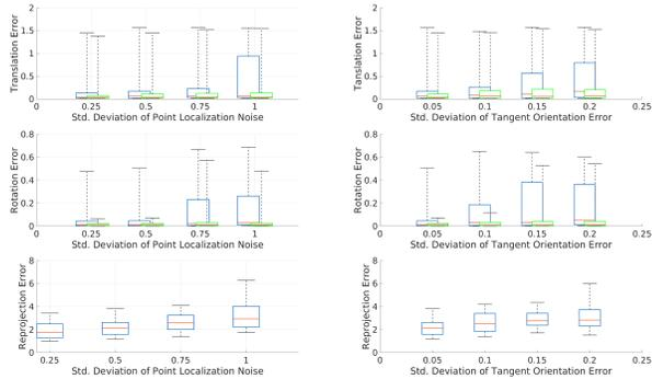
Figure 5. Distribution of trifocal pose error for the alternate formulation of Chicago in the form of translational and rotational error between cameras 1 and 2 (blue) and cameras 1 and 3 (green), as well as the reprojection error, plotted against the level of feature localization noise (left) and orientation noise (right).
