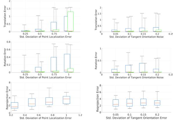
Figure 6. Distribution of trifocal pose error for the alternate formulation of Cleveland in the form of translational and rotational error between cameras 1 and 2 (blue) and cameras 1 and 3 (green), as well as the reprojection error, plotted against the level of feature localization noise (left) and orientation noise (right).
